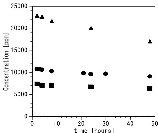
**Figure 2.** Change in the gaseous concentrations of benzene (●), tetrachloroethylene (■) and acetone (▲) in the exposure system developed. The initial concentrations are 10,700 ppm for benzene, 7,300 ppm for tetrachloroethylene and 22,800 ppm for acetone.
