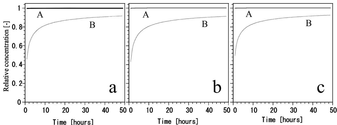
**Figure 6.** Calculated time dependency of benzene (a), tetrachloroethylene (b) and acetone (c) concentrations at the surface of the cell layer when we considered the effect of diffusion of these molecules in the surface liquid layer on the cells. The solid line (curve A) indicates the ALIC condition (the thickness of the liquid layer is 10  $\mu\text{m}$ ) and the dotted line (curve B) indicates the liquid-phase condition (the thickness of the liquid layer is 2 mm).
