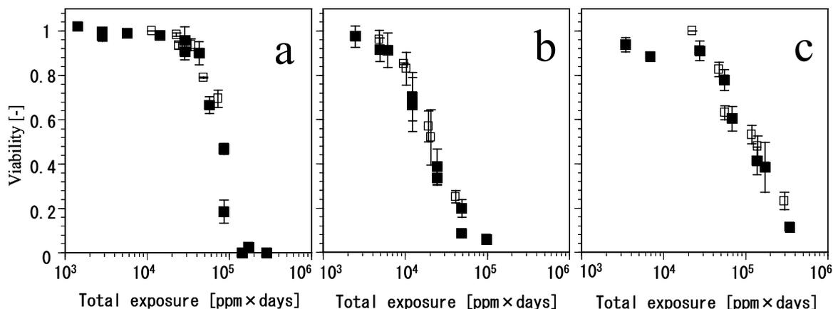
**Figure 7.** Relationship between total exposure and cell viability when loaded with benzene (a), tetrachloroethylene (b) and acetone (c) gases. The plots indicate the calculated data under the ALIC condition (■) and under the liquid-phase condition (□).
