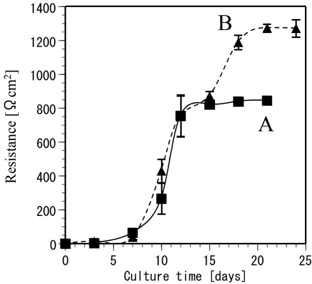
**Figure 3.** Changes in the trans-epithelium electrical resistance (TEER) of Calu-3 cells. The data was obtained from cultures in the liquid phase (■) and from cultures where the apical medium was removed after 14 days of cultivation (▲). All data subtracted the value of blank (resistance of the membrane and the culture medium), 90  $\Omega\text{cm}^2$ . All plots in the figure were the mean  $\pm$  S.D. of four wells from two independent experiments.
