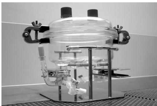
**Figure 1.** Schematic representation and photograph of the *in vitro* experimental system developed for gas exposure to cells in air-liquid interface culture (ALIC). A, Filter holder; B, Membrane filter; C, Human bronchial cells, Calu-3; D, Culture medium; E, Closed gas chamber; F, Gas sampling hole; G, Chemical substance; H, Water for humidification. This system accommodates two cell-loaded membranes under the same exposure and culture condition.
